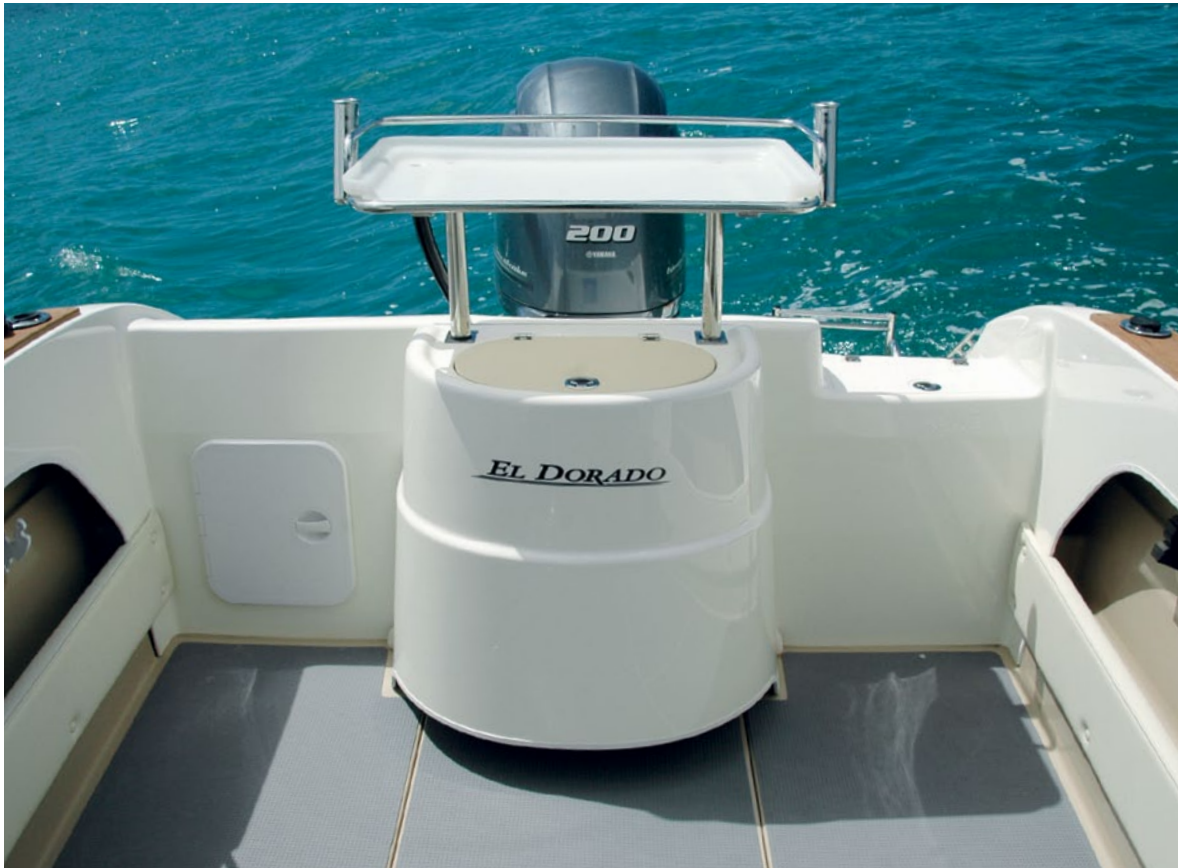
LEFT: THE CENTRAL LIVE BAIT TANK IS OPTIONAL AND LIFTS TO GIVE ACCESS TO THE BATTERIES.
