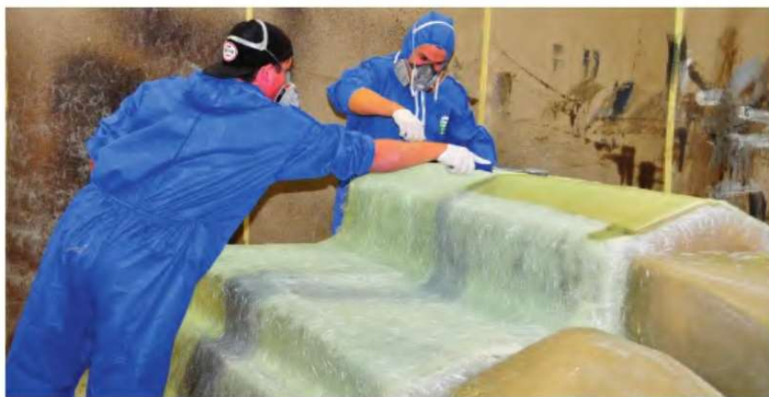
LEFT: Hand consolidation of chopper gun applied GRP. RIGHT: typical Buccaneer hull and liner join, foam filled.
