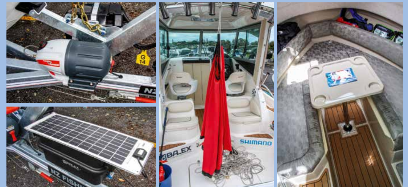
From left: Braking on both axles is provided by the AL-KO IQ7 Extreme system; A solar panel ensures the Balex ABL system is kept topped up, The Hewinson Canvas #5 sea-anchor – never leave port without it!; The cabin is suitable for overnighting in comfort. The table comes out and is replaced by an in-fill to create a double bunk.
