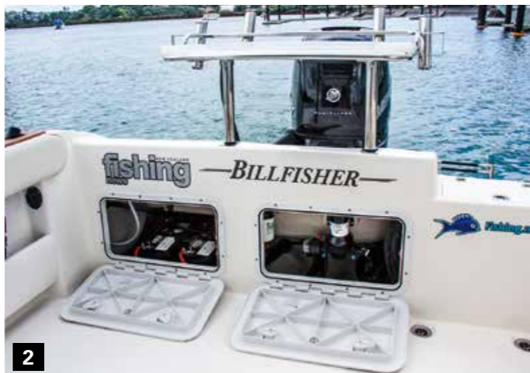
1) The large cockpit has a huge storage area under the floor, accessible via the hatch; 2) Rear hatches give access to the batteries, fuel filter and pumps; 3) Essentials such as the flare pack can be kept close at hand in the under-seat storage; 4) An Engel drawer fridge and RSE icemaker – luxury!; 5) The transom, dominated by the Mercury L6 Verado 300Hp outboard.
