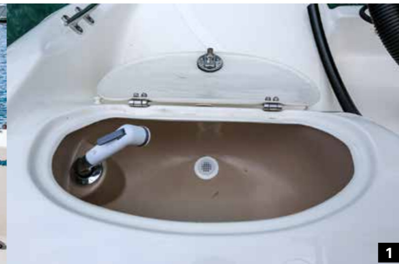
1) A freshwater shower and sink is set into the transom; 2) The forward fishing space, along with the helm-operated Maxwell RC6 capstan; 3) A feature of the Buccaneer Billfisher 735 is the full walk-around, giving easy access to the forward casting platform; 4) The Hella SeaHawk provides the illumination forward; 5) For those overnighting trips, the sink with a supply of fresh water is very handy.
