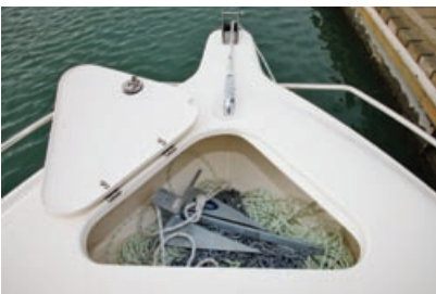
The moulded liner extends to every portion of the new 530, including the anchor locker. Underfloor stowage is generous and the compact dash is functional enough.
